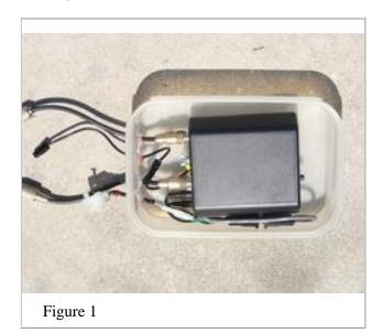
With the jumpers connected to the tuner, the extension cable and coax were run to the transceiver and the antenna erected. Now, testing was in order. The pressing of the TUNE button on my IC-706MKIIG did exactly what it was supposed to do. The Z-100 ran through its paces and signaled a good match. Now if the afternoon showers come while I am operating "fixed portable," the only
