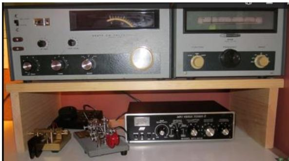
KA2F's new OLD station, Heathkit HW-16 (restored) and HG-10b VFO set up for 80, 40 and 15 meter bands, just as it was back in Novice days. The HW-16 and companion VFO are remarkably stable, after just a minute or two of warm up when compared to my Tentec Jupiter. The gear dates back to 1969. Using this station KA2F hopes to achieve WAC, WAS, and DXCC on CW, of course.
