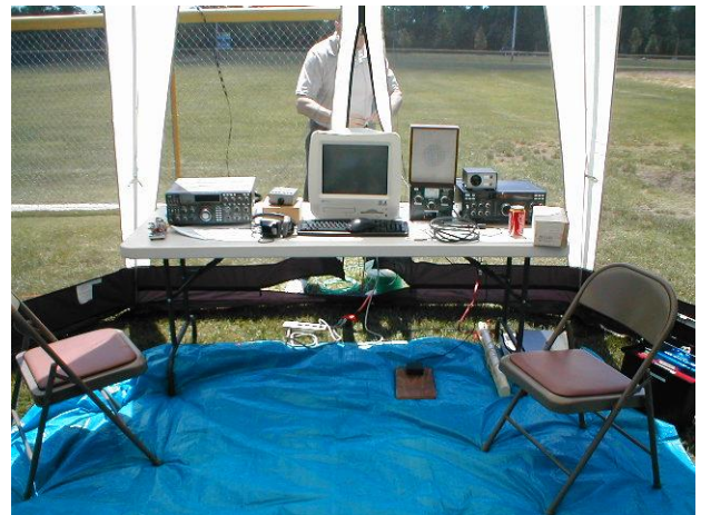
This is the operating position in the tent. The logging computer is in the center with the CW position on the left and the SSB position on the right (only one used at a time). Photo by N2LXM.
