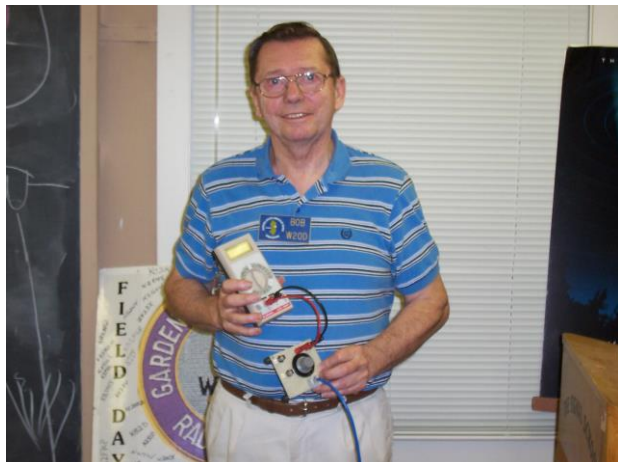
Bob, W2OD showing his cable tester with a capacitance meter (top) connected to the homebrew switch which in turn has a piece of RJ-45 Ethernet cable under test dropping down out of the picture. Photo by Ray, W2NXG.
